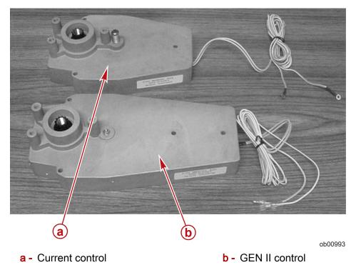
NOTE: The new GEN II controls must use new GEN II throttle and shift cables.
